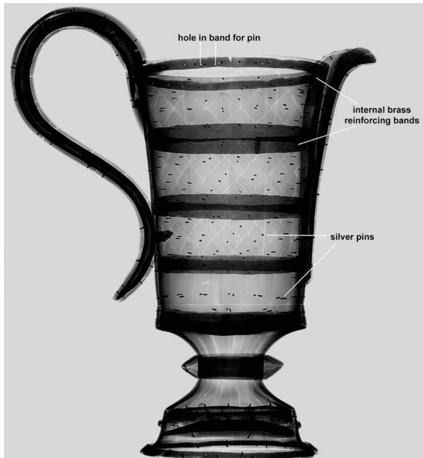
FIGURE 4. X-radiograph (negative image) of an ewer. The darkest areas are the densest: note the reinforcing bands. The concave shape just above the rim of the foot is a valve of a *P. margaritifera* shell
