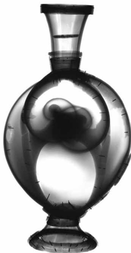
FIGURE 7. X-radiograph (negative image) of the bottle, OA+ 2642. The pins are very long and the construction appears comparatively crude
