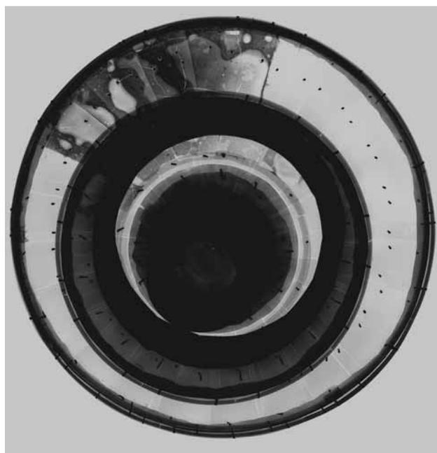
FIGURE 6. X-radiograph (negative image) of candlestick OA+ 2644 taken from above showing an area of patchy adhesive on the flared base, similar to that on the other candlestick. The dark circle in the centre is the candle socket, and the dark ring around this is the wall of the base seen from above. Note that the candlestick has been constructed slightly off-centre
