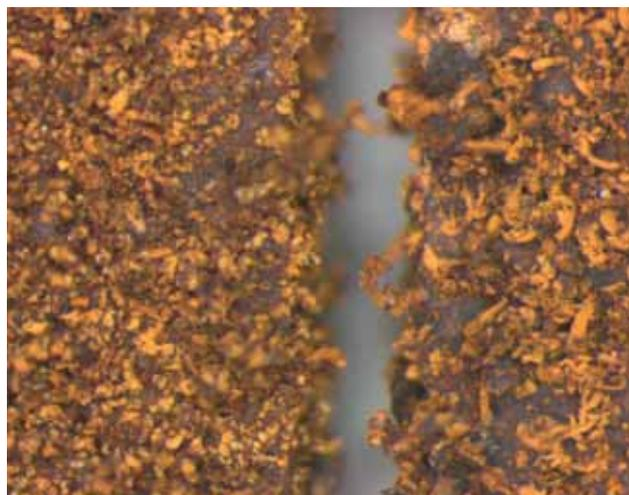
FIGURE 8. Stereo microphotograph of control foils exposed at 54% RH for six months, showing akaganéite formed on the industrial iron (left) was less developed than that formed on wrought iron (right). Image width: 3.5 mm
