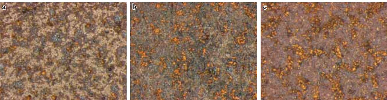
FIGURE 7. Stereo microphotograph of three control foils after four weeks exposure at 54% RH: (a) industrial iron in a sealed chamber; (b) wrought iron in a sealed chamber; (c) industrial iron in a chamber with two holes. Width of each image: 3.5 mm
