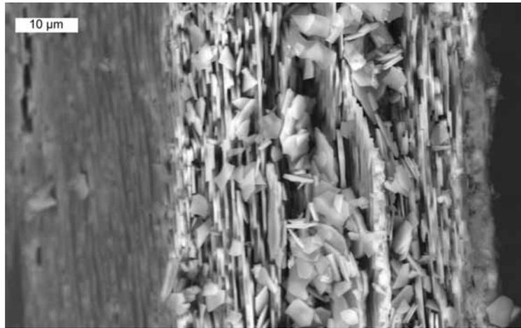
FIGURE 4. Scanning electron microscope (SEM) image of the laminated, friable microstructure of *Pinctada* mother of pearl oyster shell
