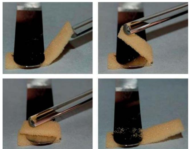
**Figure 8. Testing the flexibility of the foam samples to assess the effects of varying the treatment time**
