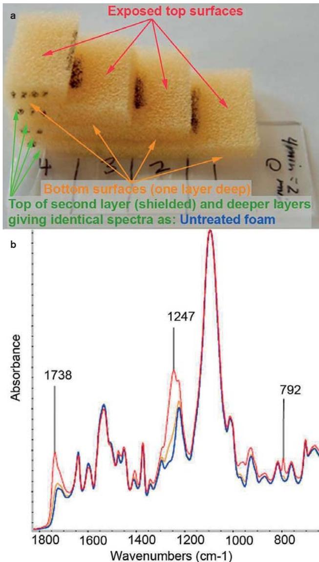
**Figure 9.** Analysis of the stepped foam layers using ATR-FTIR to test the depth of penetration: (a) the locations at which measurements were made; and (b) the spectra recorded at these locations. The red spectra were recorded on the top surfaces exposed to the consolidating mist, the yellow spectra on the bottom surface of the layer exposed to the mist, the green spectra on the bottom surfaces deeper in the layer structure and the blue spectra on untreated foam
