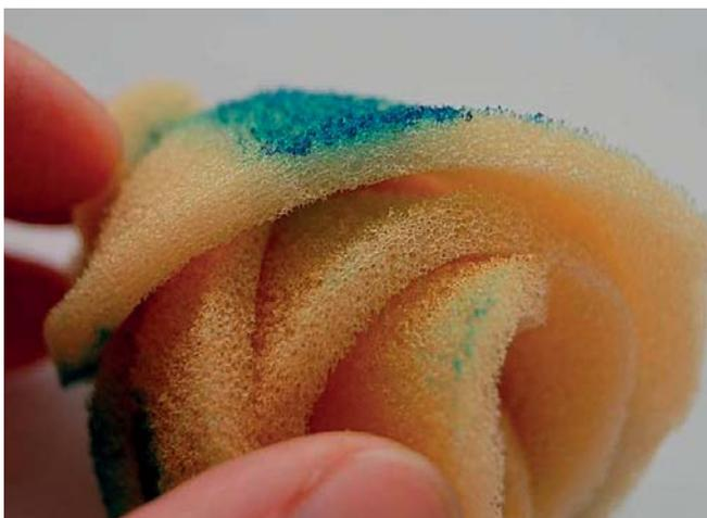
**Figure 10.** Foam rose model treated with a consolidant mixture containing methylene blue as an indicator
