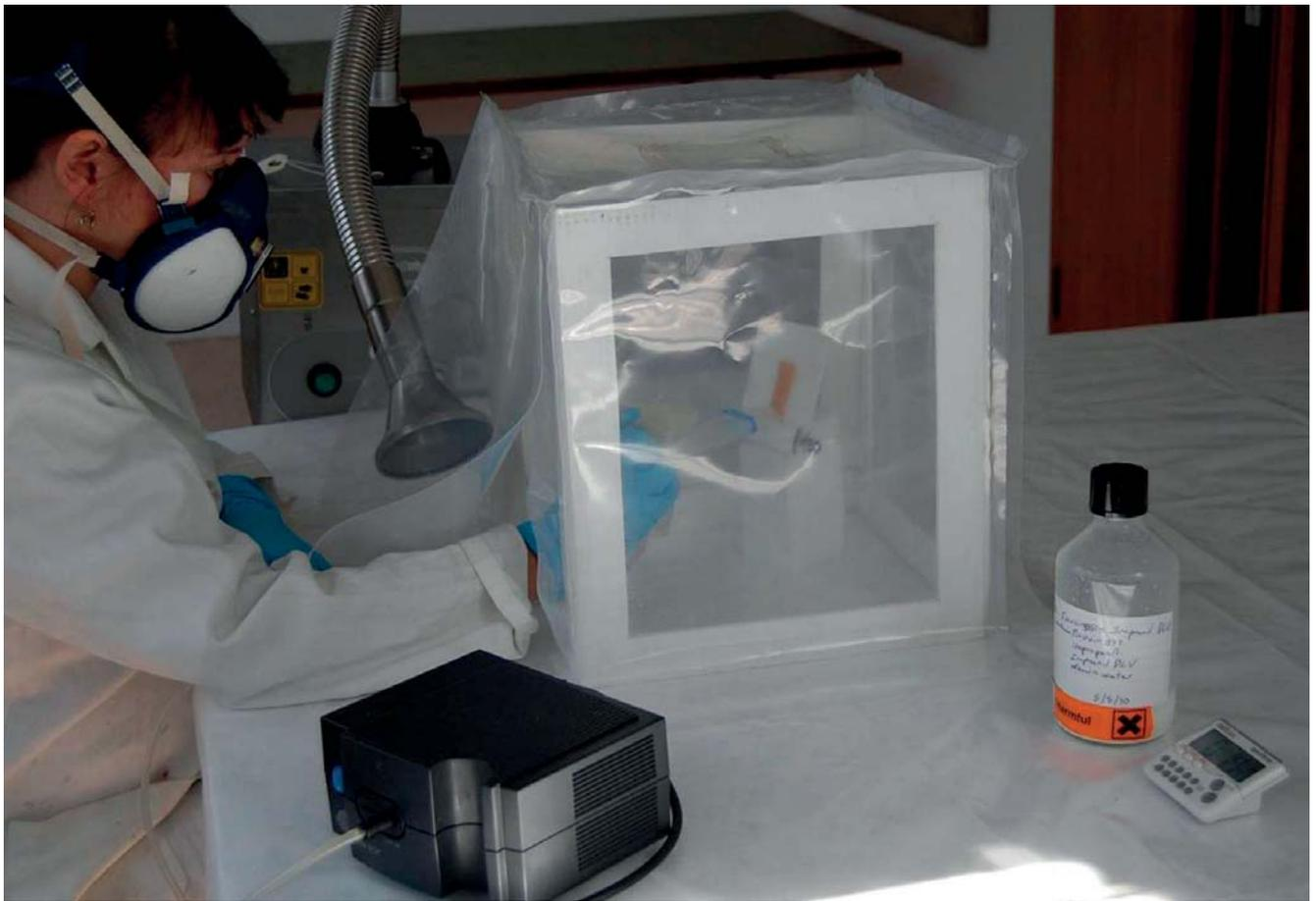
**Figure 7. Treating a sample of aged foam with the nebulizer inside a custom-made enclosure**
