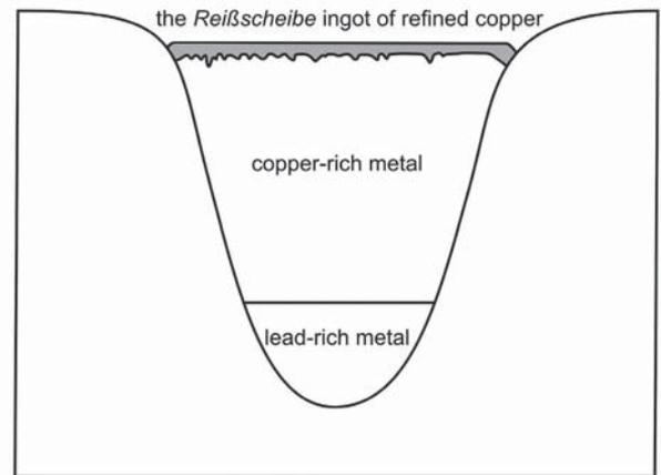
FIGURE 4. Diagram showing the principle of the *Reifsscheibe* refining process
