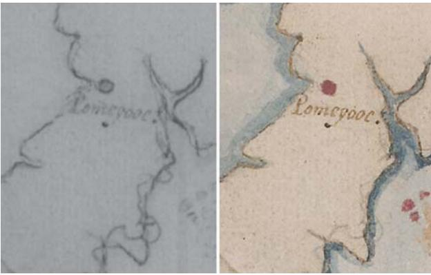
FIGURE 6. Area to the east of Lake Paquippe showing changes between the initial sketching, as shown in the infrared reflectogram (IRR; left) and the finished map, as shown in the reflected visible light image (right). Once alerted by the IRR image many of the changes can be seen by eye
