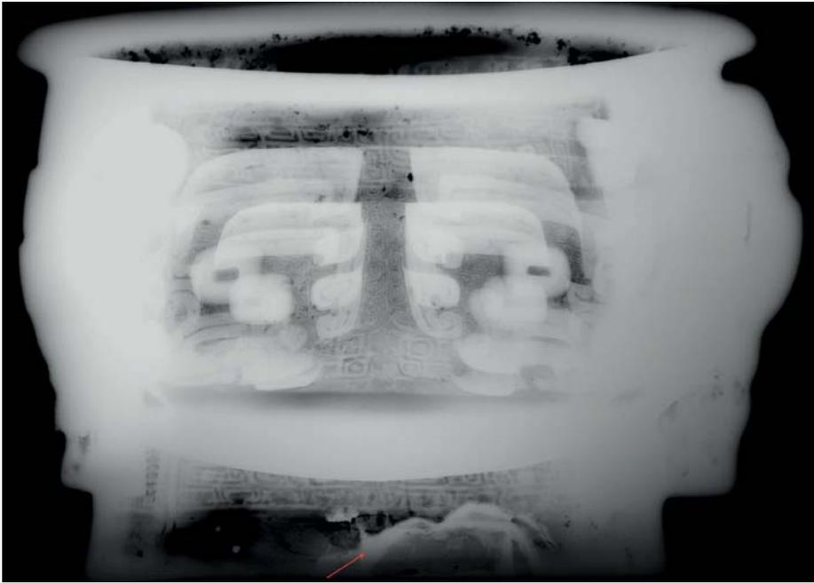
FIGURE 3. X-radiograph of the vessel showing repairs on the foot (indicated by an arrow) and the dark spots in the region of the rim that indicate porosity in the casting
