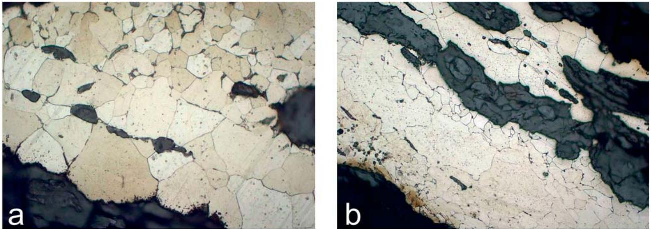
FIGURE 6. Scanning electron micrographs of samples from the kettle-hat: (a) sample SN1086 from the crown of the helmet showing slag inclusions, larger ferrite grains near the surface and small quantities of intergranular pearlite between the smaller ferrite grains; and (b) sample SN1087 from the rim of the helmet showing small slag inclusions, corrosion (large dark area) and bands of different-sized ferrite grains containing minute carbide or carbo-nitride precipitates. Width of field: 0.68 mm
