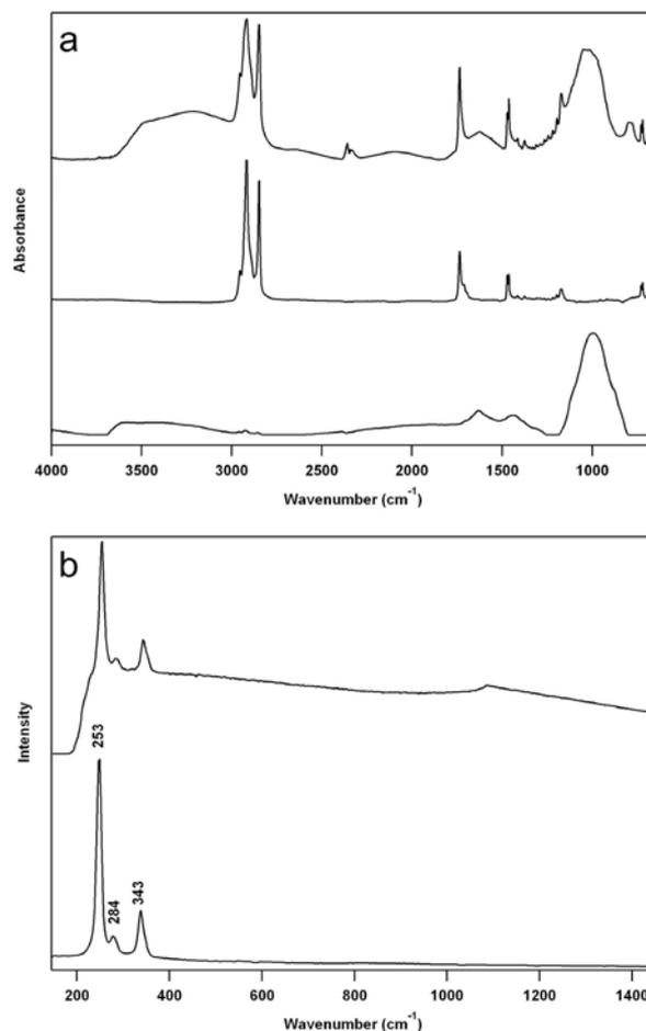
FIGURE 2. The identification of samples from the helmet: (a) ATR FTIR spectra of a sample of a mixture of waxy and green materials taken from the surface (upper trace), a reference sample of beeswax (middle trace) and a reference sample of siliceous green earth (lower trace); and (b) Raman spectra of a sample of red material from the surface (upper trace) and a reference sample of vermilion (lower trace)
