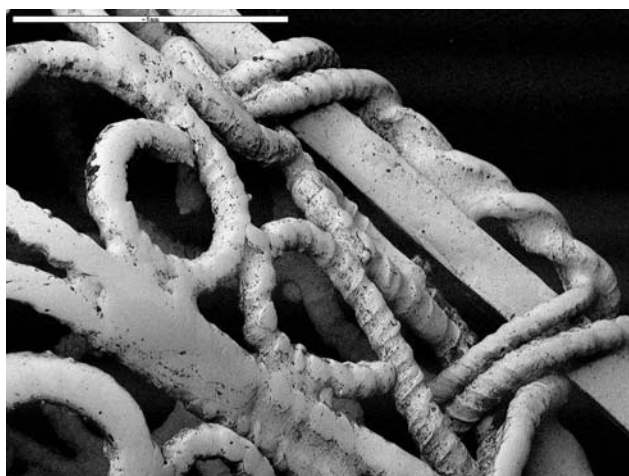
FIGURE 3. Avar gold earring (1933,0405.13); SEM detail with thin spiral beaded wire with decoration soldered in place. Note the extensive wear on the exposed regions of the gold. Scale bar: 5 mm
