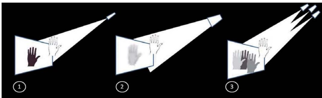
FIGURE 4. The influence of hologram illumination on the holographic image: (1) a narrow beam spotlight where the light is generated from a very small area gives a sharply focused hologram; (2) a spotlight with a wider light source size that illuminates the hologram gives a more blurred image; and (3) multiple light sources give rise to a series of holograms
