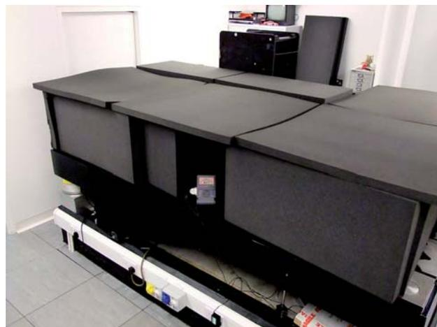
FIGURE 5. The recording room at CMO, which is adjacent to the laser room. The heavy table floats on air cushions, while the recording area is surrounded by polyethylene foam blocks that isolate the object from air turbulence. The power meter at the centre is used to measure the light emitted from the lasers
