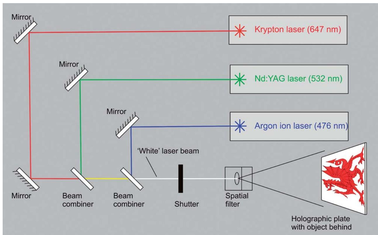
FIGURE 2. Experimental configuration used to record colour reflection holograms
