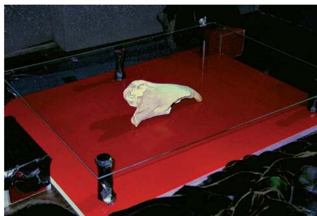
FIGURE 6. The Kendrick's Cave horse jawbone set up for holography on the red surface of the recording table
