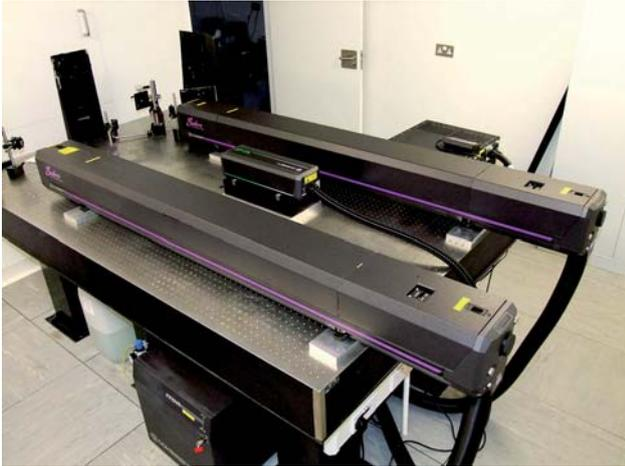
FIGURE 3. The red krypton laser, the green Nd:YAG laser and the blue argon laser in the laser room at CMO
