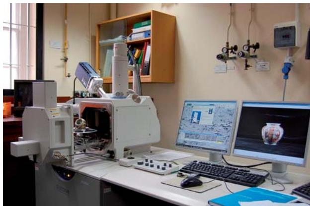
FIGURE 4. The Hitachi S-3700N Variable Pressure SEM used for the porcelain examination. The large jar is on the sample stage ready to be inserted into the very large sample chamber. The analytical X-ray detector is the blue device on the left side of the chamber. There are two large high-resolution imaging screens, one displaying the visible image of the pot
