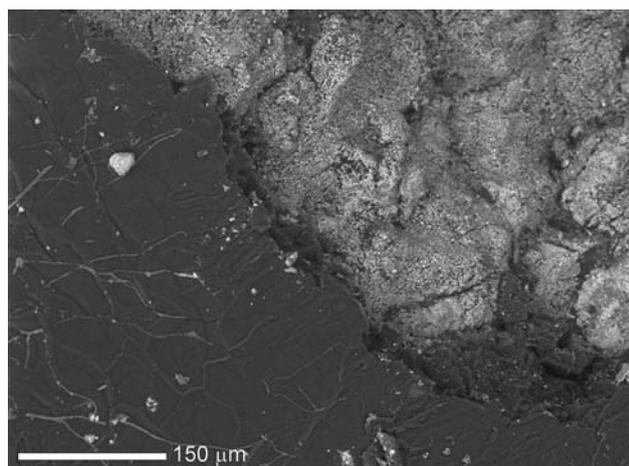
FIGURE 9. An unprovenanced sample of Jericho wood, showing thick wax deposits to the lower left and the area cleaned by the laser to the upper right. Image: Hitachi TM-1000 SEM
