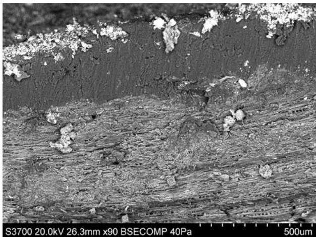
FIGURE 4. Backscattered electron image of a tangential longitudinal section through a table fragment made from *Cedrus libani* (cedar of Lebanon) wood, showing the soil present in the surface wax layer and the extent to which the wax has penetrated into the cellular structure. Image: Hitachi S-3700N VP-SEM
