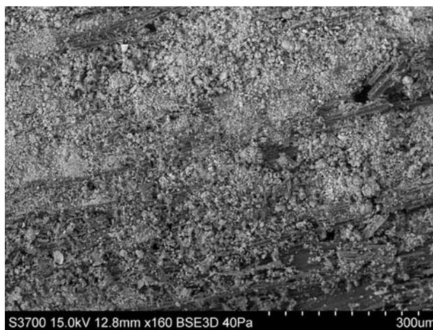
FIGURE 7. Backscattered electron image of a tangential longitudinal surface of a fragment from an artefact, showing loose pieces of wood, detritus and soil present in the surface wax layer. Image: Hitachi S-3700N VP-SEM
