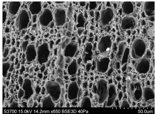
FIGURE 5. Backscattered electron image of a transverse surface of a fragment from a wooden artefact from P19 made of *Crataegus* sp. (hawthorn), showing severely shrunken and distorted vessels, fibres and parenchyma cells. Image: Hitachi S-3700N VP-SEM
