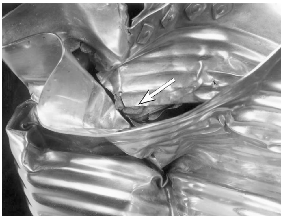
Plate 11 Detail of inside of cup showing a lower outer rivet head through a tear
