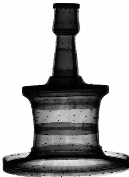
FIGURE 5. X-radiograph (negative image) of candlestick OA+ 2643. Note the patchy areas on the base (bottom left) and on the neck just below the candle socket. These appear to be a denser adhesive, perhaps indicative of a repair
