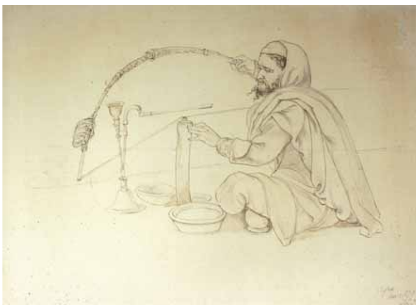
FIGURE 3. Pencil and ink drawing by John Lockwood Kipling of a lapidary at Agra, India, 1870, using a traditional wire saw to cut a small stone mounted on a post. One end of the bow was hand held whilst the opposite end was balanced with a weight; the wire was charged with an abrasive mix from the bowl. Drawing (0929/52) is reproduced by kind permission of Victoria and Albert Museum, London
