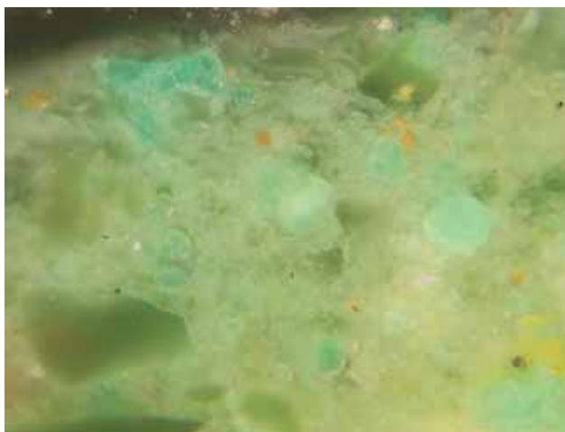
FIGURE 2. Cross-section of a sample from the 'green' block, clearly showing the mixture of organic and inorganic materials
