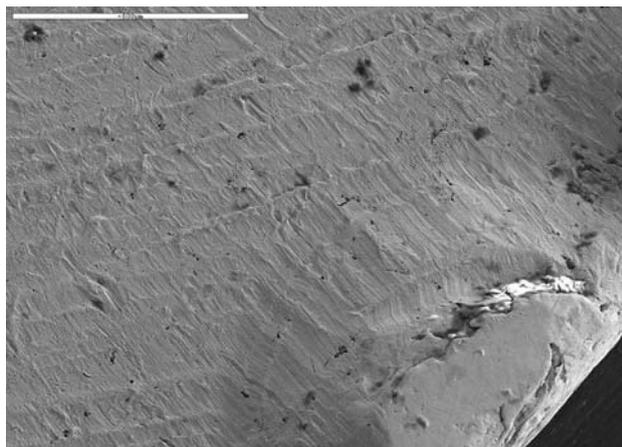
FIGURE 3. Secondary electron image in the SEM of the gold mancus of Coenwulf, showing striations on the edge beading due to die striking. Scale bar length 500  $\mu\text{m}$
