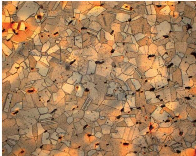
FIGURE 3. Photomicrograph of a polished section of the ring (No. 11) showing an annealed structure; etched with ethanolic iron(III) chloride. Image width: 0.27 mm
