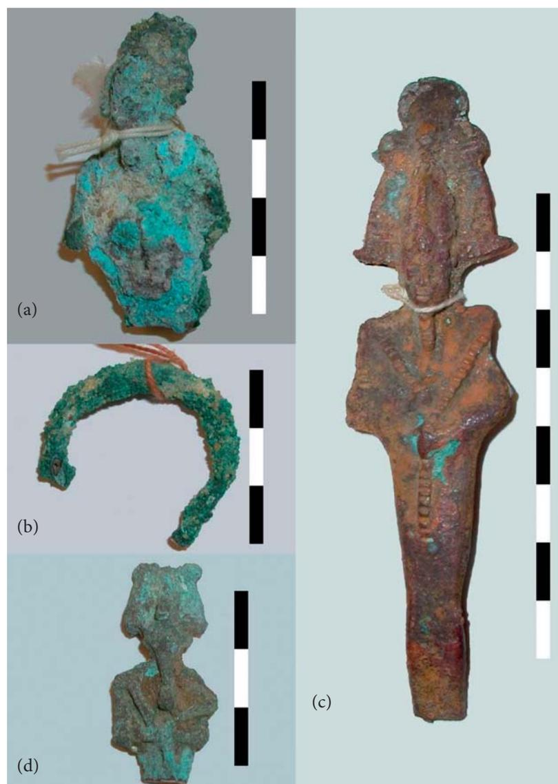
FIGURE 1. Four objects from which samples were taken for metallographic study in cross-section: (a) torso of Osiris, No. 8; (b) ring, No. 11; (c) Osiris, No. 12; and (d) Osiris, No. 14. Scale bars show 1 cm divisions
