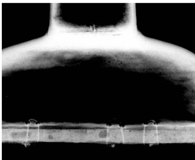
FIGURE 6. Detail of the X-radiographic image of the joint between the top and bottom sections of the ewer. The overlap where the two sections fit together appears as the pale band across the image. The wire (white) is threaded through the pair of holes in the upper section and re-emerges from the pair of holes in the lower section, where the ends of the wire were twisted together. All this is now concealed on the exterior by enamel
