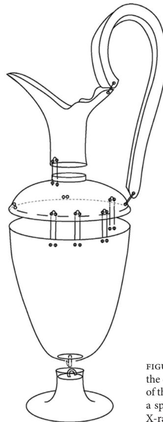
FIGURE 4. X-radiographic image of the ewer and an exploded diagram of the metal construction based on a speculative interpretation of the X-radiographs
