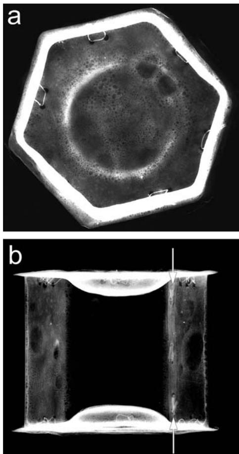
FIGURE 2. X-radiographic images of the salt cellar: (a) top view and; (b) side view showing the strip metal 'stitches' running down the side (marked with arrows) and the thin wire loops (white) threaded through holes in the top and bottom to hold them in place
