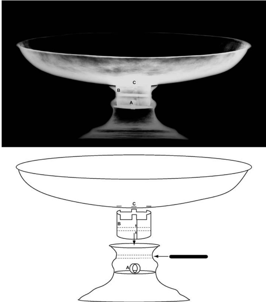
FIGURE 9. X-radiographic image of the footed bowl (note that the hollow foot does not quite touch the bottom of the bowl) and an exploded diagram of the metal construction as interpreted from the X-radiographs: 'A' is the enamelled disc with loop; 'B' the metal cylinder with stitched seam; and 'C' the bowl pierced by four slots to take the four tabs on the top of the metal cylinder
