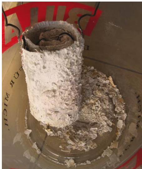
Figure 5 Lead white has formed as flakes on a lead coil, which was exposed to vinegar fumes and carbon dioxide for about a month (reconstruction by Carmen Krisai-Chizzola).
